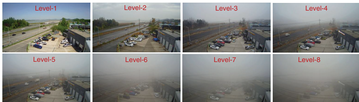
Figure 5: Examples of CCTV images labelled with eight different visibility levels
