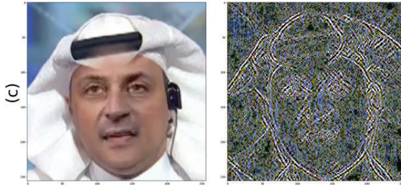
Figure 3: Noise feature extracted by the High-frequency Noise Extraction Module from (a) authentic face and face manipulated by (b) Deepfakes and (c) FaceSwap
