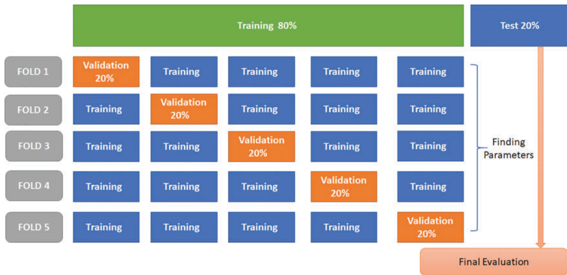
Figure 2: Illustration of the K-fold cross-validation scheme with an 80–20 training-testing split and 20% of each fold used for validation to optimize model parameters before final evaluation
