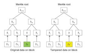
Figure 1: The second preimage attack on the block based on Merkle Tree
