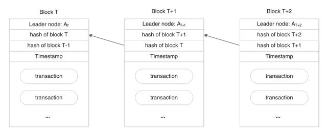
Figure 6: Structure of quantum-enhanced blockchain
