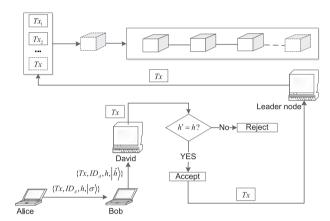
Figure 5: Transaction process in quantum-enhanced blockchain
