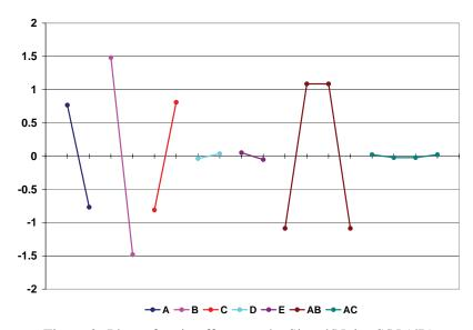
Figure 2: Plots of main effects on the Signal/Noise S/N (dB).
