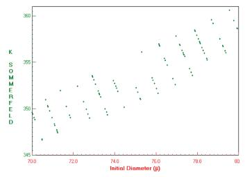
Figure 4: Scatterplot of the Sommerfeld number vs. initial particle diameter. Simulation made on the code *Jets&Poudres*.
