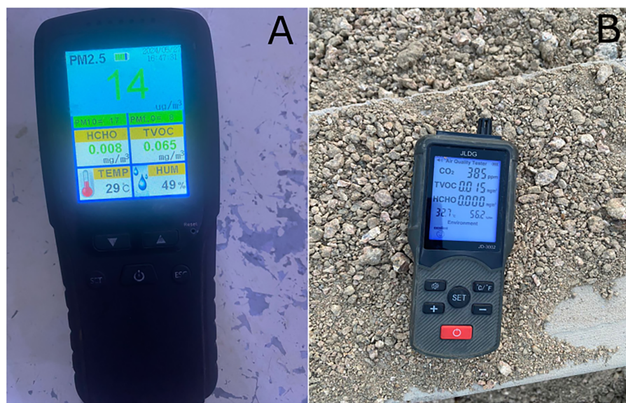
Figure 3: (A) DM106A air quality monitor, and (B) JD-3002 professional air quality meter.
