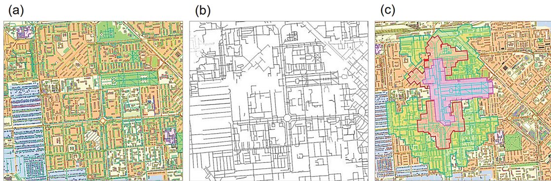
Figure 1: Spatial network graph and pedestrian accessibility to park based on municipal GIS data: (a) GIS data, encompassing sidewalks, pedestrian pathways, and street networks; (b) constructed routing graph; (c) network distances to the park—830 m (10 min walk), 1250 m (15 min walk), and 1785 m (21 min walk)
