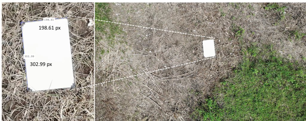
Figure 7: Computation of the Ground Sampling Distance (GSD) used a reference marker with known dimensions, which provides the equivalent ground distance (in centimeters) per pixel in the image. The GSD computed is 0.1 cm/px
