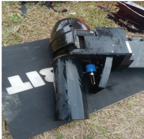
Figure 2: Multibeam echosounder system used in this study (NORBIT iWBMS MBES)
