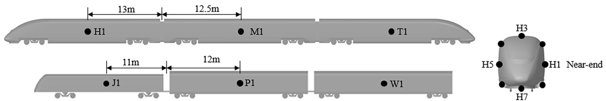
Figure 10: Schematic diagram of surface pressure measurement points on passenger and freight trains.
