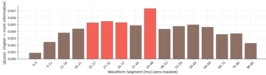
Figure 6: Loss sensitivity to zero-masking 16 waveform segments. Highlighted bars (top 25% sensitivity) peak at 27–32 ms and 43–48 ms, consistent with 1–2 bearing fault impulse repetition periods at the target operating speed (BPFO \approx 107 Hz).
