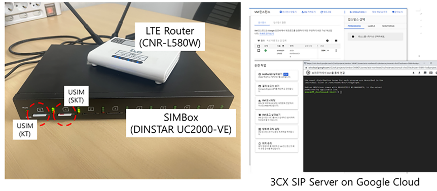
Figure 4: Experimental SIMBox call environment: SIMBox and LTE router ( left ), and the 3CX SIP server deployed on Google Cloud Platform ( right ).
