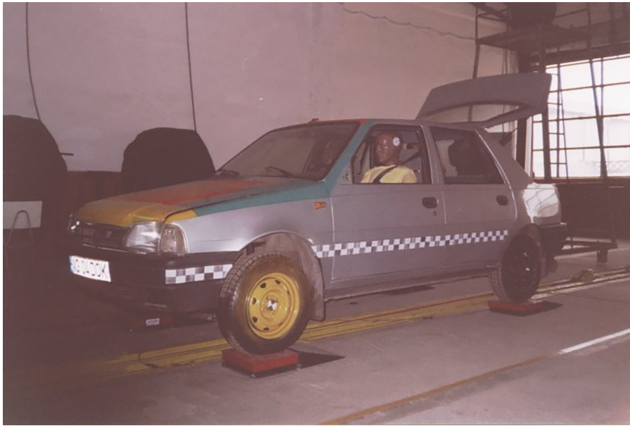
Figure 15: Delimitation of areas with different potential for injury on the front surface of the vehicle.
