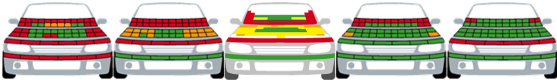
Figure 16: Level of injury to pedestrians by the front surface of a car, evolution over time (adapted from EuroNCAP).
