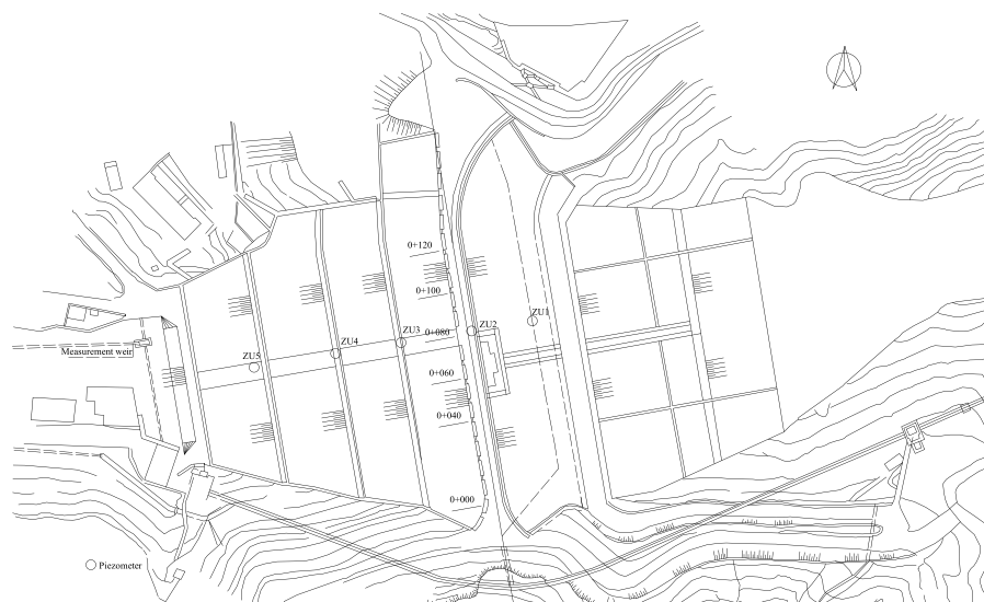
Figure 3: Location plan of seepage monitoring points and the gauge weir on the main dam.
