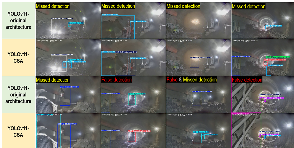
Figure 7: Comparison of construction element recognition performance between the two models.
