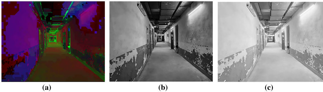
Figure 4: Adaptive brightness adjustment results of the value (V) channel. (a) HSV image; (b) value (V) channel; (c) adaptive value (V) adjustment.
