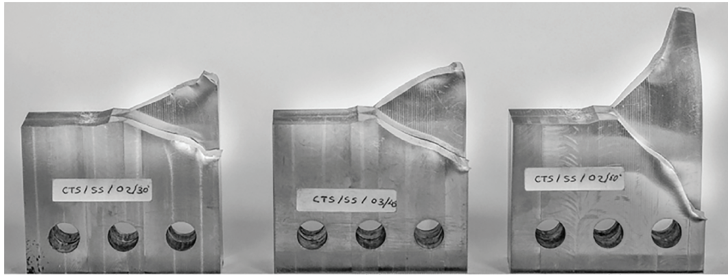
Figure 11: Experimental crack growth path: (a) 30° loading angle [49], (b) 45° loading angle [49], and (c) 60° loading angle [49]
