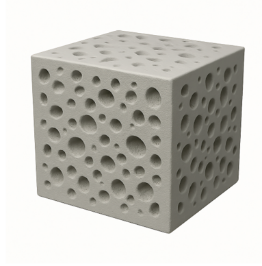
Figure 7: Porous medium model with randomly distributed spherical pores
