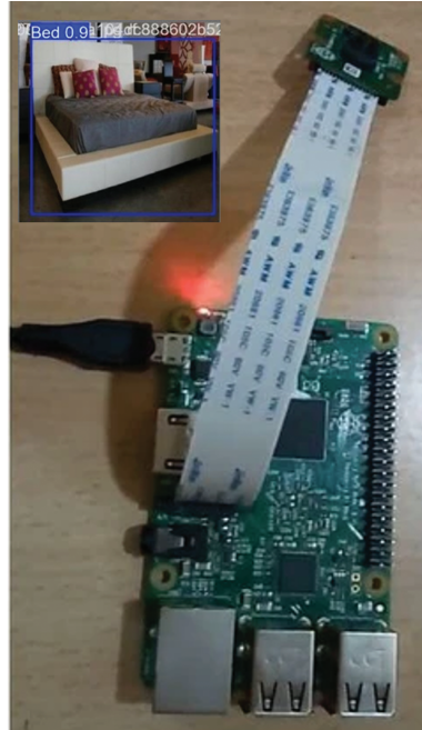
Figure 2: The Raspberry Pi connection with the wearable IoT device for indoor object detection assistant
