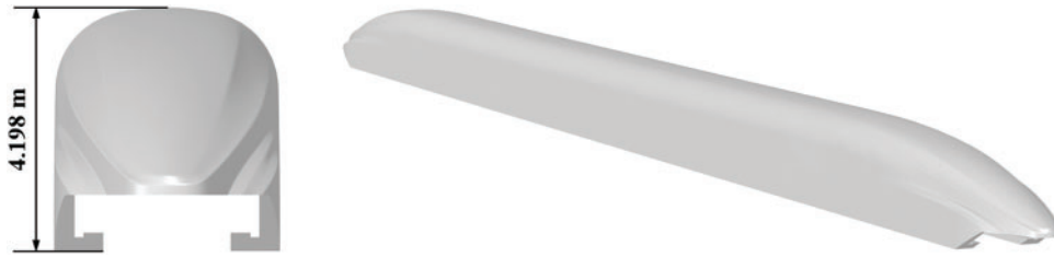
Figure 5: Train geometry model used for numerical verification
