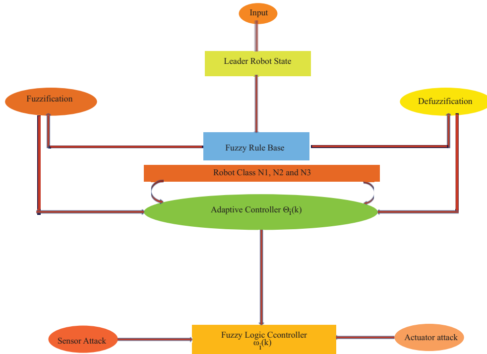
Figure 4: Block diagram of the fuzzy logic-based robust control framework under sensor and actuator attacks
