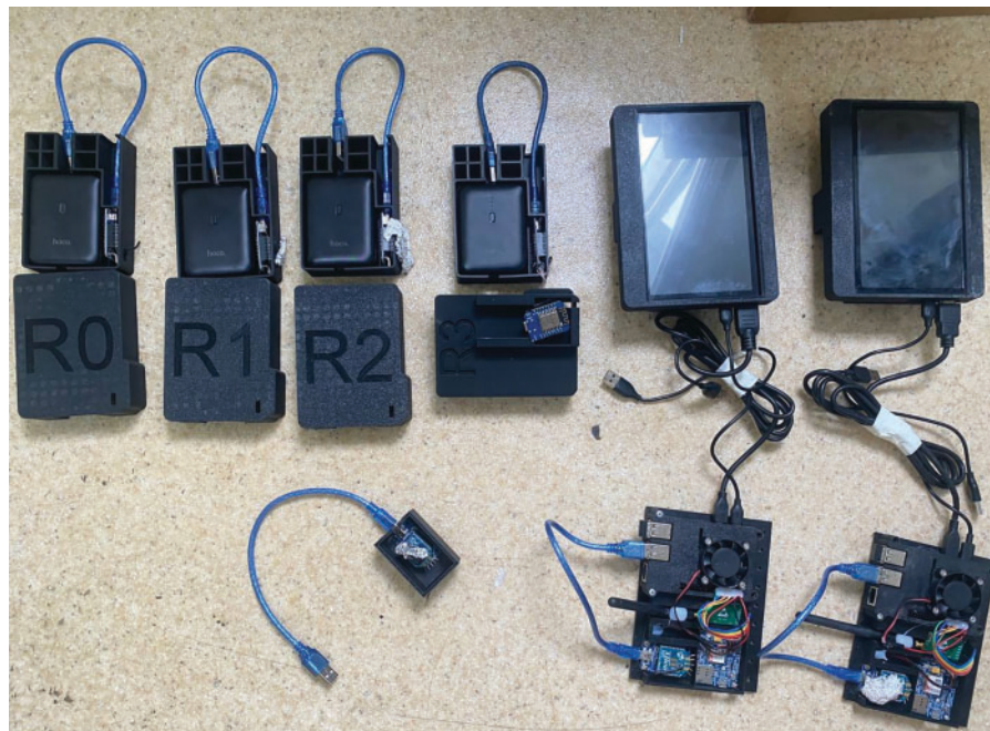
Figure 4: The simulated WSN node of with the router role
