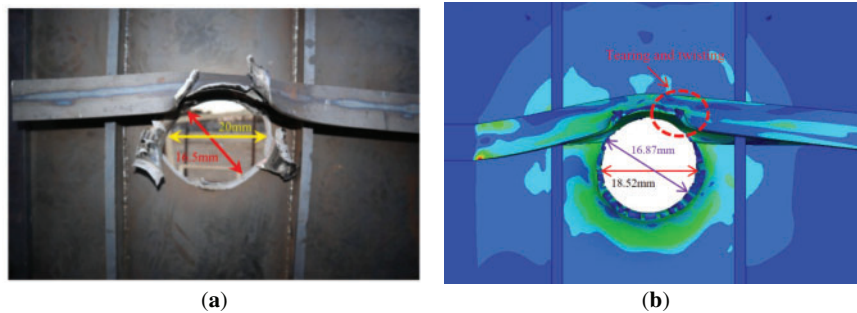
Figure 9: The comparison between experimental and numerical result of stiffened plate suffering projectile penetration. (a) Experimental result of Wang et al. [35]; (b) Numerical result
