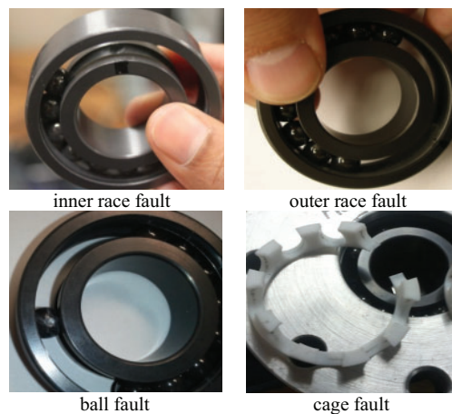
Figure 5: Bearing seeded faults
