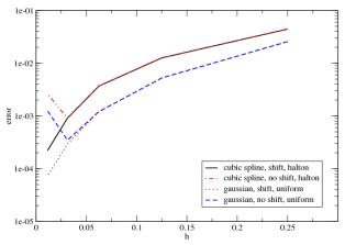
Figure 6: Errors raised solving problem  $\mathcal{P}_M$ , using either shifted (dashed lines) or non shifted (solid lines) polynomial basis functions.
