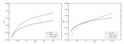
Figure 2: Problem  $\mathcal{P}_D$ , errors raised when exploiting uniform discretizations. We set  $\beta = 2.5$ , q = 2 (left frame), q = 3 (right frame).
