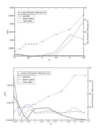
Figure 1: Errors raised solving problem  $\mathcal{P}_D$ , when  $\beta$  parameter changes;  $\alpha=1$  was set. The finest uniform grid,  $U_5$ , was exploited. Either Gaussian or spline weights are enrolled. A quadratic GMLS basis (q=2) is exploited in the top frame; A cubic one (q=3) is exploited in the bottom frame. The maximum number of non–zero values per row in the final coefficient matrix is also shown.
