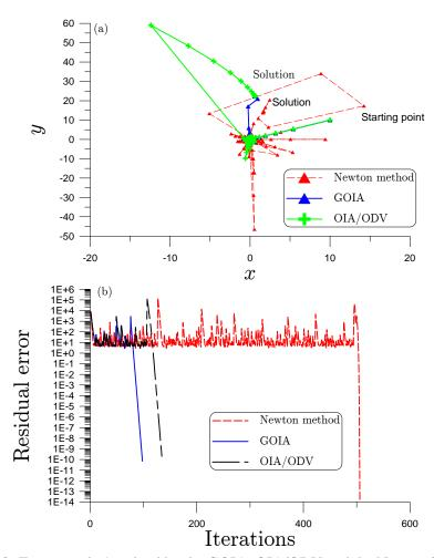
Figure 2: For example 1, solved by the GOIA, OIA/ODV and the Newton iterative, comparing (a) the solution paths, and (b) the residual errors.
