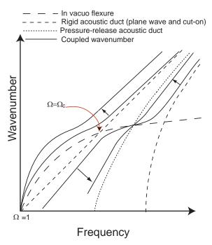
Figure 9: Schematic of the coupled wavenumber solutions. Arrows indicate the transition of solutions as  $\varepsilon$  increases.
