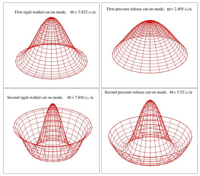
Figure 2: Cut-on acoustic modes in cylindrical duct for the axisymmetric mode (n = 0).
