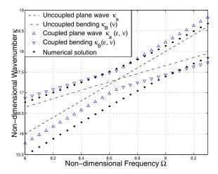
Figure 7: Coupled wavenumber solution near the coincidence frequency for the fluid-filled infinite cylindrical shell with h/a=0.1,  $c_L/c_f$ =2,  $\varepsilon$ =0.2 and v = 0.25, vibrating in the axisymmetric mode.
