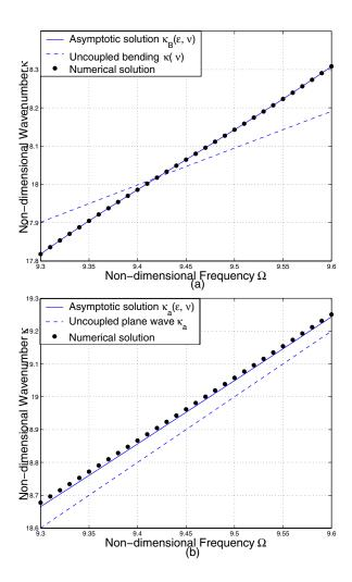
Figure 8: Coupled wavenumber solution above the coincidence frequency ( $\Omega_c$ ) for the fluid-filled infinite cylindrical shell with h/a=0.1,  $c_L/c_f$ =2,  $\varepsilon$ =0.2 and v = 0.25, vibrating in the axisymmetric mode (a) for the bending wave (b) for the acoustic plane wave.
