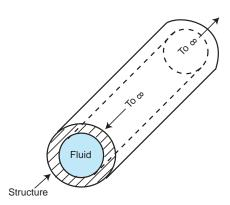
Figure 1: Schematic of the model showing the fluid-filled flexible cylindrical shell of infinite length.
