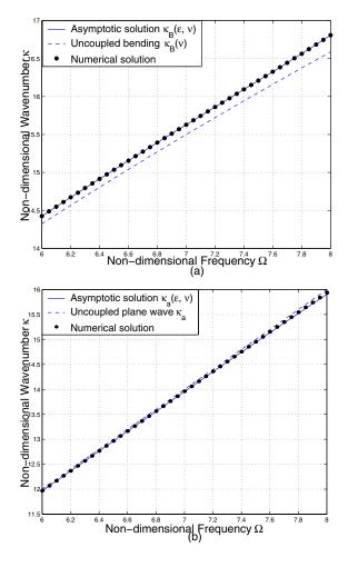
Figure 6: Coupled wavenumber solution below the coincidence frequency ( $\Omega_c$ ) for the fluid-filled infinite cylindrical shell with h/a=0.1,  $c_L/c_f$ =2,  $\varepsilon$ =0.2 and v = 0.25, vibrating in the axisymmetric mode (a) for the bending wave (b) for the acoustic plane wave.
