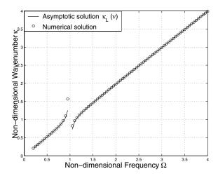
Figure 3: Wavenumber corresponding to the dominantly longitudinal mode obtained through the asymptotic method and the numerical solution for v = 0.25 and h/a = 0.05.
