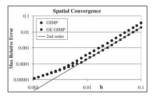
Figure 13: 1D Improvement due to Gradient Enhancement
