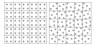
Figure 1: Ideal Versus General Particle Positions
