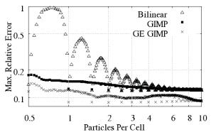
Figure 12: 1D Solution Accuracy with Increasing PPC
