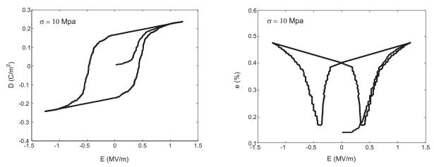
Figure 7: Hysteresis and butterfly curves under quasi-static loading with lateral compressive stresses  $\sigma = 10 \text{ MPa}$ .
