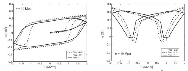
Figure 9: Hysteresis and butterfly curves under axial compressive stresses  $\sigma = 10$  MPa for  $\hat{E} = 2.0$  MV/m.
