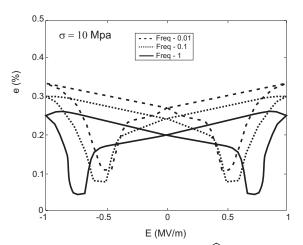
Figure 17: Hysteresis and butterfly curves under lateral compressive stresses  $\sigma = 10$  MPa for  $\hat{E} = 1.0$  MV/m.
