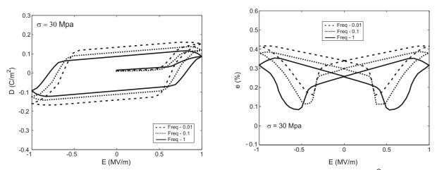
Figure 20: Hysteresis and butterfly curves under lateral compressive stresses  $\sigma = 30$  MPa for  $\hat{E} = 1.0$  MV/m.
