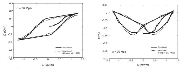
Figure 6: Hysteresis and butterfly curves under quasi-static loading with axial compressive stresses  $\sigma = 30 \text{ MPa}$ .
