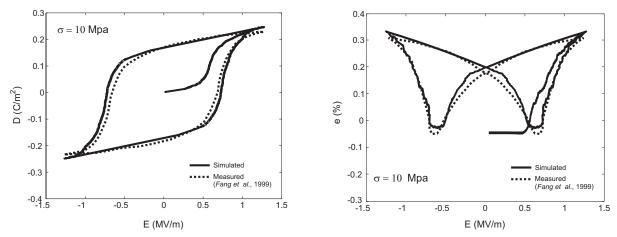
Figure 5: Hysteresis and butterfly curves under quasi-static loading with axial compressive stresses  $\sigma = 10 \text{ MPa}$ .
