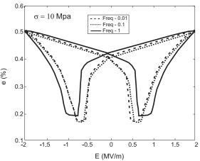
Figure 15: Hysteresis and butterfly curves under lateral compressive stresses  $\sigma = 10$  MPa for  $\hat{E} = 2.0$  MV/m.
