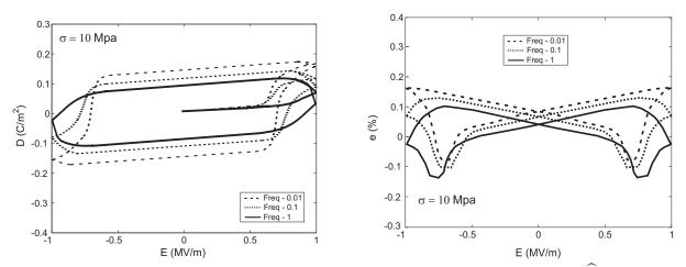
Figure 11: Hysteresis and butterfly curves under axial compressive stresses  $\sigma = 10$  MPa for  $\hat{E} = 1.0$  MV/m.
