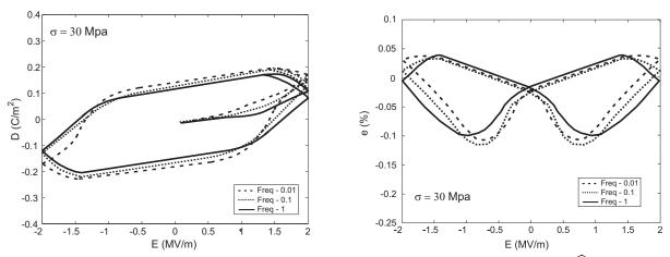
Figure 12: Hysteresis and butterfly curves under axial compressive stresses  $\sigma = 30$  MPa for  $\hat{E} = 2.0$  MV/m.
