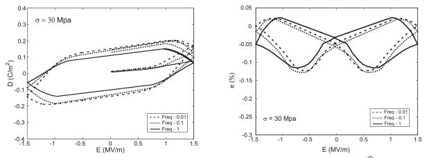
Figure 13: Hysteresis and butterfly curves under axial compressive stresses  $\sigma = 30$  MPa for  $\hat{E} = 1.5$  MV/m.
