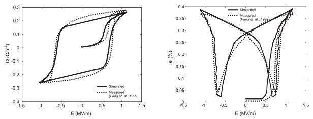
Figure 4: Hysteresis and butterfly curves under quasi-static loading with probabilistic approach (p = 5) but without additional superimposed stresses.
