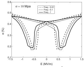
Figure 16: Hysteresis and butterfly curves under lateral compressive stresses  $\sigma = 10$  MPa for  $\hat{E} = 1.5$  MV/m.
