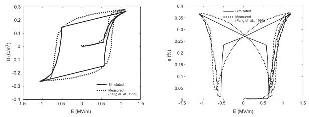
Figure 3: Hysteresis and butterfly curves under quasi-static loading without probabilistic approach (p = 0) and without additional superimposed stresses.
