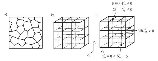
Figure 2: Two-dimensional graphical representation of a natural assembly of grains (a), schematic three-dimensional finite element discretisation (b), and illustration of the applied boundary conditions (c).
