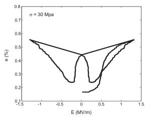
Figure 8: Hysteresis and butterfly curves under quasi-static loading with lateral compressive stresses  $\sigma = 30 \text{ MPa}$ .
