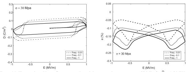
Figure 14: Hysteresis and butterfly curves under axial compressive stresses  $\sigma = 30$  MPa for  $\hat{E} = 1.0$  MV/m.
