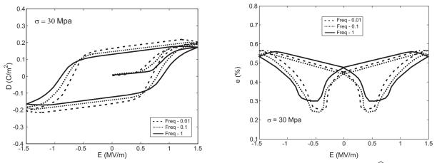
Figure 19: Hysteresis and butterfly curves under lateral compressive stresses  $\sigma = 30$  MPa for  $\hat{E} = 1.5$  MV/m.
