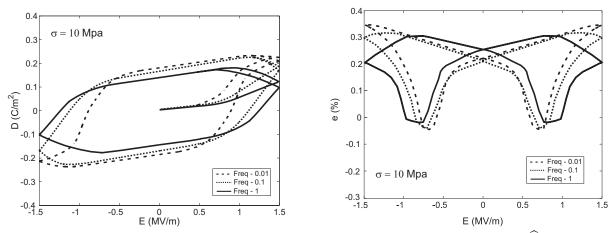
Figure 10: Hysteresis and butterfly curves under axial compressive stresses  $\sigma = 10$  MPa for  $\hat{E} = 1.5$  MV/m.
