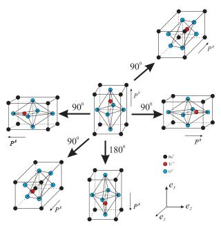
Figure 1: Different types of 90° and 180° domain switching for a representative tetragonal lattice structure.
