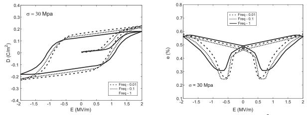
Figure 18: Hysteresis and butterfly curves under lateral compressive stresses  $\sigma = 30$  MPa for  $\hat{E} = 2.0$  MV/m.
