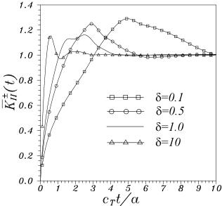
**Figure 11**: Effects of the anisotropy parameter  $\delta$  on  $\overline{K}_I^{\pm}$  and  $\overline{K}_{II}^{\pm}$ -factors
