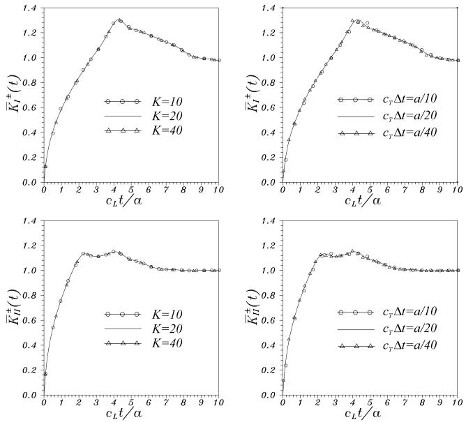
**Figure 3**: Effects of the truncation limit K on  $\overline{K}_I^{\pm}$ - and  $\overline{K}_{II}^{\pm}$ -factors ( $c_T \Delta t = a/20$ , isotropic solids)
