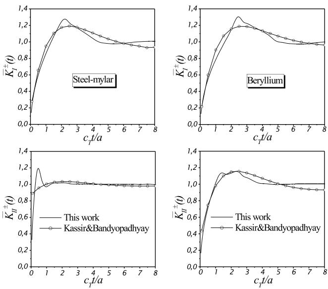
**Figure 9** : Normalized  $\overline{K}_{I}^{\pm}$  - and  $\overline{K}_{II}^{\pm}$ -factors
