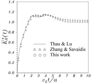
**Figure 2**: Normalized  $\overline{K}_I^{\pm}$ - and  $\overline{K}_{II}^{\pm}$ -factors (isotropic solids)
